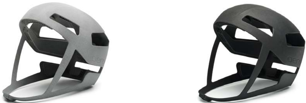
Figure 5. HP Multi Jet Fusion printed part before (left) and after dyeing (right)
