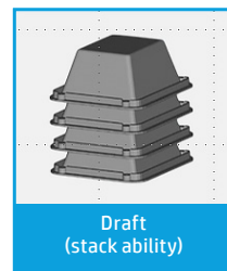
Figure 13: Optimized use of the build volume
