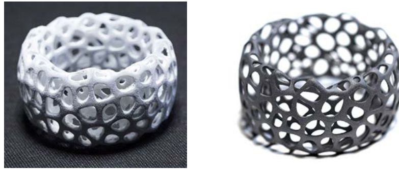
Figure 2. Part after unpacking, uncleaned (left); Part after cleaning (right)
