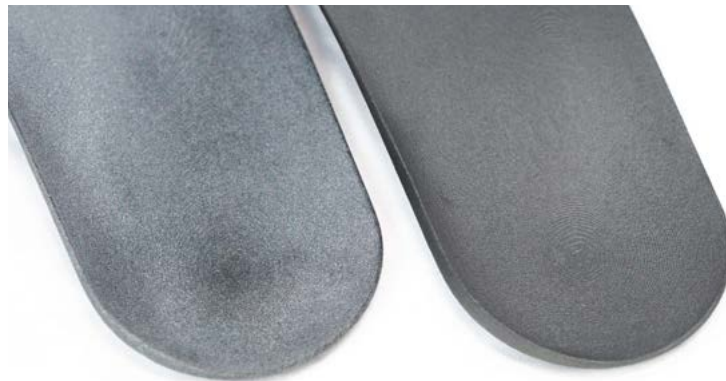
Figure 6. Printed part cleaned with glass beads (left); part cleaned with metal media (right)
