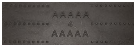
Figure 4. Dyed part with scratch marks (left) that are removed by using bead blasting (right)
