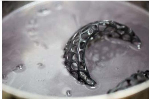
Figure 3. Dyeing process of HP Multi Jet Fusion printed parts
