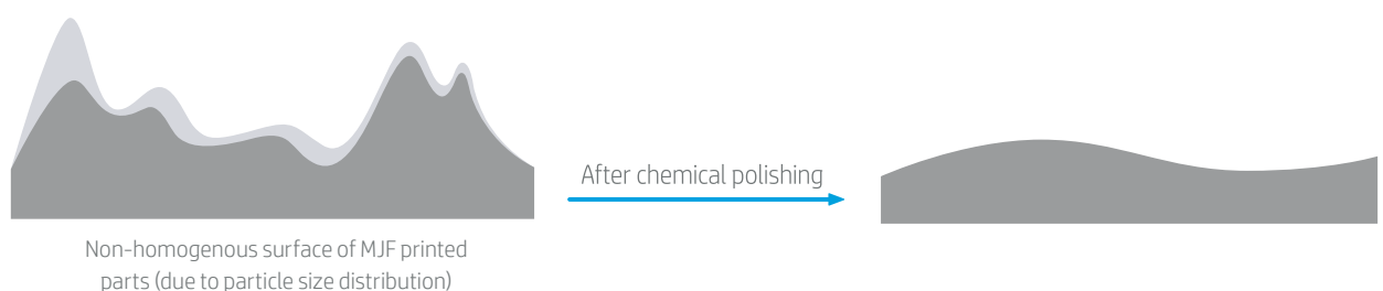
Figure 15. Surface roughness improvement after chemical polishing
