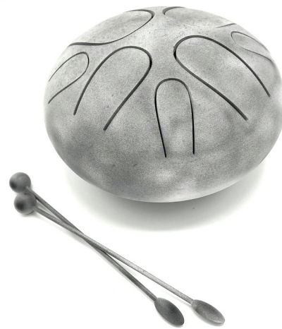
Figure 2: Large hollow parts with reasonably thin walls and holes can create a nice resonance. In the example above, the cut-out "tongues" on the drum act like cantilevers. The tone they generate is a function of the mass of the cantilever and is therefore controlled by thickness, length, shape, and cross section
