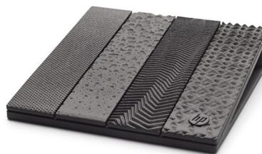
Figure 12: Example of texture to increase adhesion
