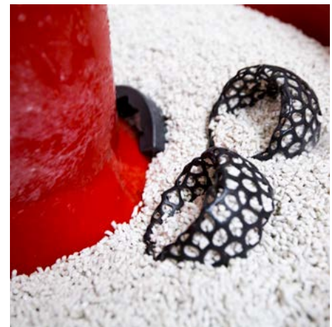
Figure 13. Printed parts being processed in the tumbler
