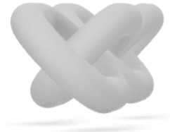
Figure 9: Chain links oriented at -45 and +45 degrees to the print bed
