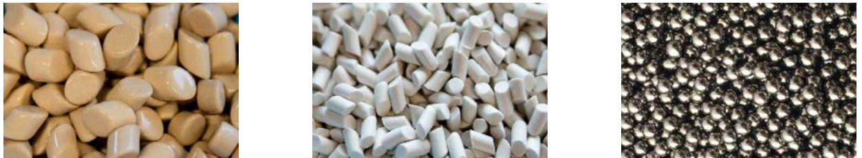
Figure 14. Different blasting media used in tumbling process: ceramic, plastic, and steel (from left to right)
