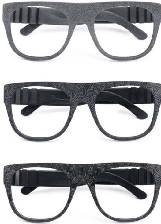
Figure 16. Image of raw part, and two chemically polished parts with varying degrees of processing
