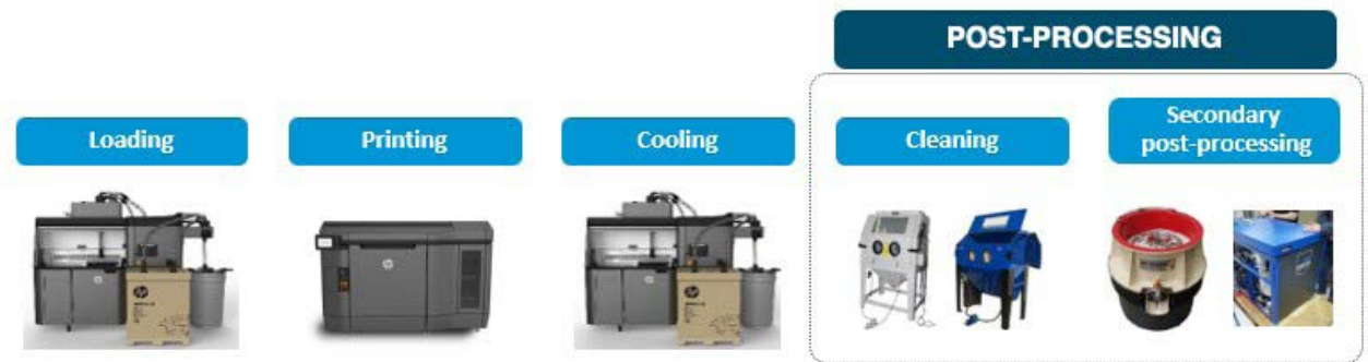
Figure 1. E2E HP Jet Fusion 3D Printing workflow
