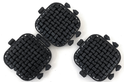
Figure 3: Another type of hinge uses cones that fit into matching divets. These modules can snap apart and back together.
