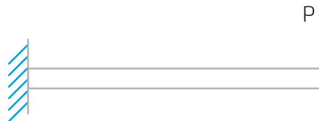
Figure 10. Cantilever beam with a point-applied end load
